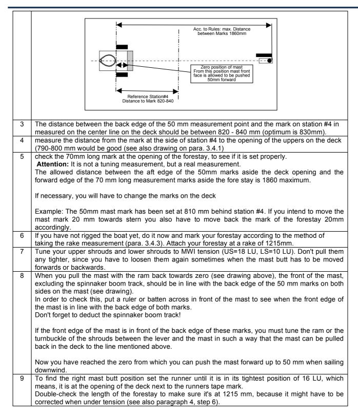
**Remember:** The maximum tension of the runners at a rake of 1215mm is at 16 LU. This runner tightening procedure seems to be very rough at first, but if your Dragon can't take it while at the dock without waves or wind pressure, something will certainly break while sailing.
